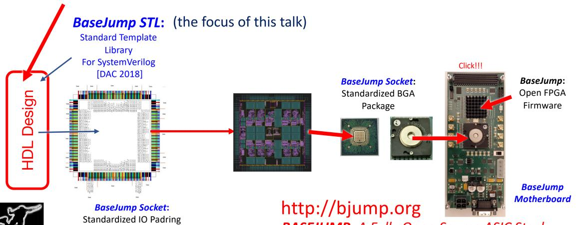
**BASEJUMP:** A Fully Open-Source ASIC Stack
